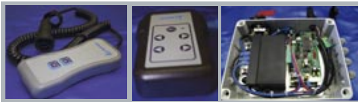
The boxtron system (box above) can be supplied in "tele" or "radio" (wireless) control. In this case, the box cover includes the "radio" device.
