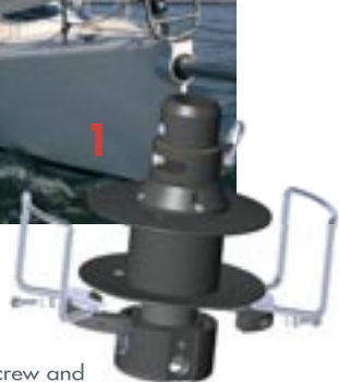
1 Unscrew and remove the furling line guide
