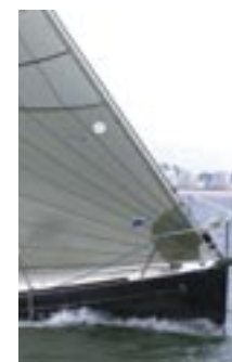
4 Once the half plates are removed, a racing Genoa can be hoisted using the twin groove head foil
