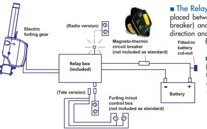
■ The Relay box is a polarity inversing gear that is placed between the power supply (battery + circuit breaker) and the drive unit. It inverses the rotation direction and therefore enables to furl in or out. the Fitted-in foil sections turn at constant speed
