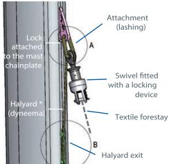
\* Halyard partially without outer shell on 1.1 to 1.2x the luff length
