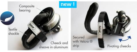
Four models from 2 to 7 tons (SWL): 2T/ 3T / 4T5 / 7T CNC machined cheecks (black anodized) and the sheave (colorless anodizing) offer a light design and resistance. Moreover, the composite bearing lowers the risk of corrosion. No specific maintenance require.
