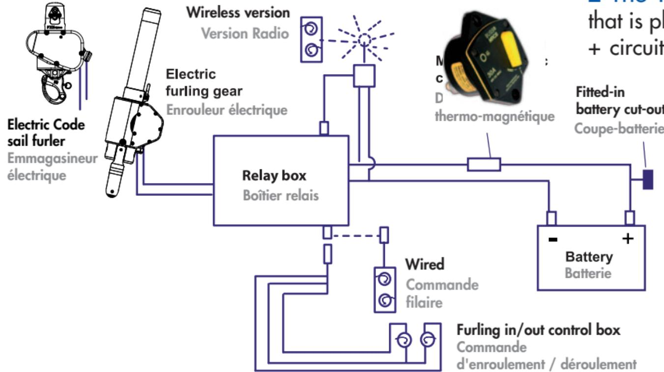
■ The **Relay box** is a polarity inverting gear that is placed between the power supply (battery + circuit breaker) and the drive unit. It inverts the rotation direction and therefore enables to furl in or out. the foil sections turn at constant speed
